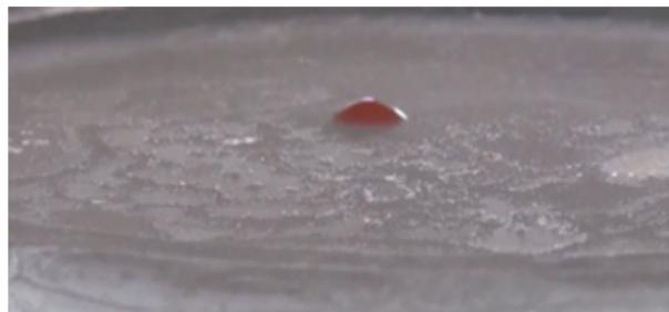
Fig. 3: 9 seconds after water drop depositing on the plate.
