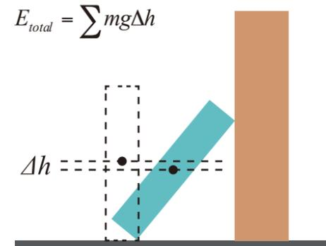
Fig 1. The block released gravitational potential energy through its center of gravity dropped  $\Delta h$ .
