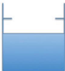
Fig.7. using a baffle to ignore splashing
