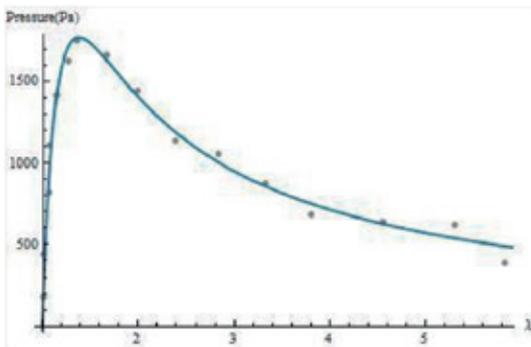
Diagram 2. Pressure vs. Extension. At first by inflating air pressure increases and reaches a peak but the volume increases hence pressure decreases.
