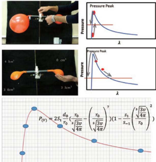
Diagram 7. P-λ: in two small and big balloons connected to each other. Red points are related to the initial condition of two balloons.
