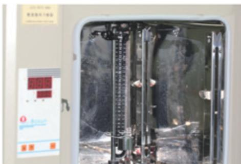
Fig.4. GZX-9140MBE Electro-thermostatic blast oven
