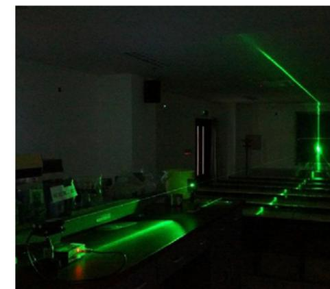
Fig. 2. Experiment setup, which shows the semiconductor laser (bottom left), optical slit (middle) and the blackboard (right).
