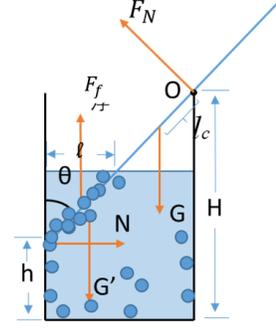
FIG. 2. Diagram of mechanical analysis of straws in carbonated drink.
