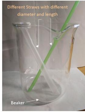
FIG. 3. Image of the experimental device for the straws in carbonated drink.
