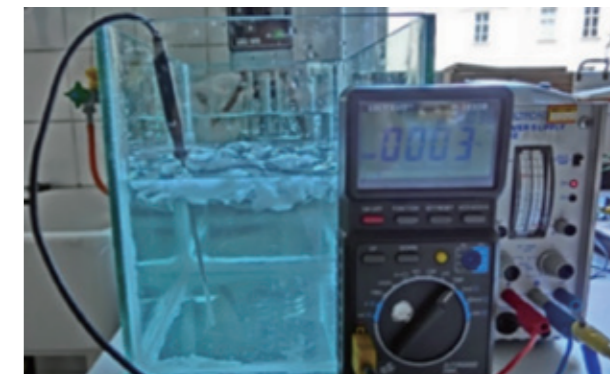
Figure 7: Cooling bath to shock cool the cocoa butter and to analyse how many phase changes may occur when shock cooling.
