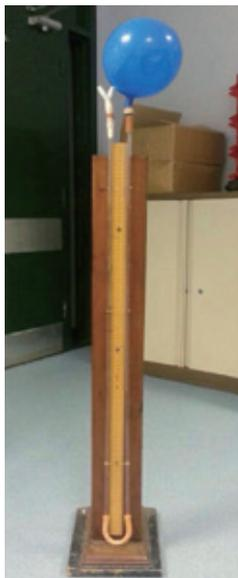
Fig.2. A water manometer is used to measure the excess pressure inside the balloon.
