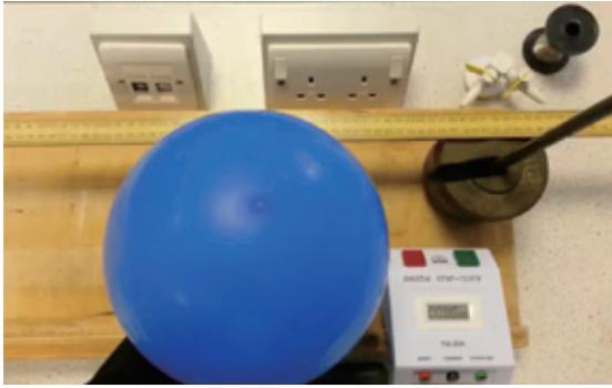
Fig.5. We filmed the process of deflation, and then we analysed the video to determine the diameter of the balloon.
