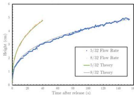
FIG. 8. Height of the conical pile for different nozzle radius (cm) versus time (sec) after release.
