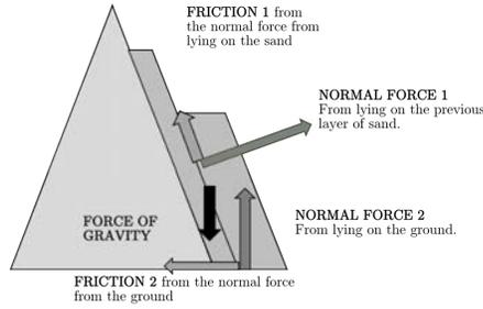
FIG. 9. Free body diagram on two discrete layers on a sand pile.
