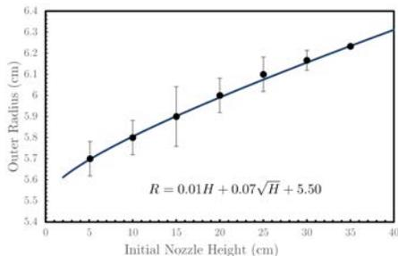
FIG. 6. The outer radius of the conical pile during formation versus the height of the nozzle.
