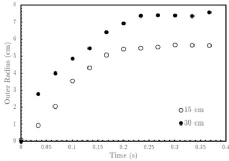
FIG. 5. Outer radius of the conical pile during formation versus time for two different initial heights.
