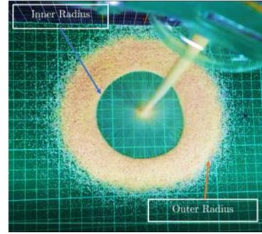
FIG. 3. The formation of the bottom of the conical pile.
