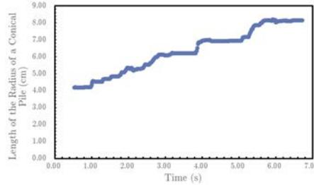
FIG. 7. The Growth of a 200 g conical pile, dropped from 10 centimeters above.
