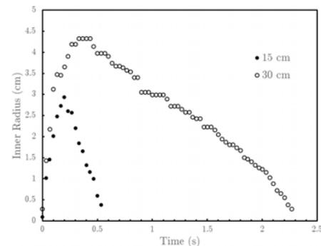
FIG. 4. Inner radius of the conical pile during formation versus time for two different initial heights.
