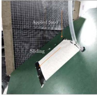
FIG. 1. Experimental Apparatus to test the angle of repose of a granular system.
