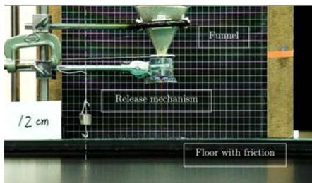
FIG. 2. Experimental apparatus of measuring the shape of the conical pile.
