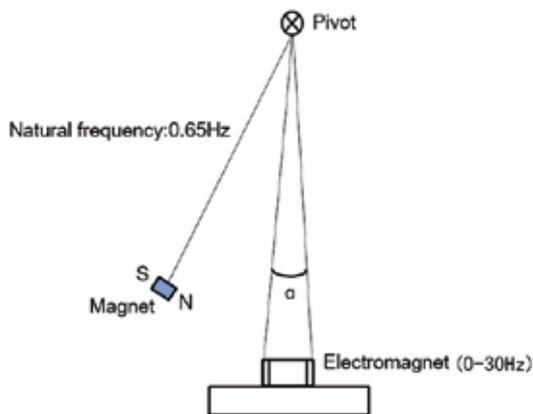
Fig.1. Diagram of magnetic pendulum. The moment of inertia of the pendulum is  $0.064/\text{kg}\cdot\text{m}^2$ . Natural frequency is about  $0.65\text{Hz}$ . Magnetic pole of permanent magnet is marked in Fig.1.
