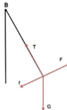
Fig.2. Force analysis diagram. The pendulum is forced by gravity, magnetic force, friction and tension.
