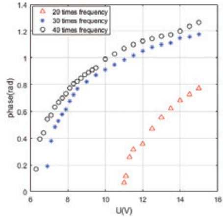
Fig.12. if  $f_1 = n f_2, n=20,30,4$ , phase will be locked in different value by changing U (V). The explanation for phase locking is still tenable, since Phase and U shows positive correlation while Phase and frequency shows positive correlation.
