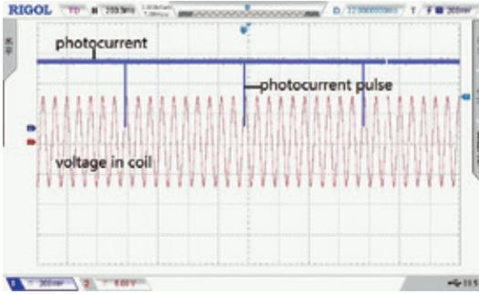
Fig.7. The frequency relationship between photocurrent and voltage in coil.
