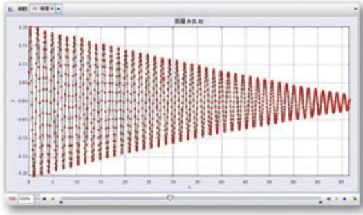
Fig.4. Decayed oscillation without kick-up by electromagnet.
