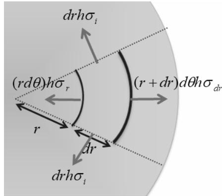
FIG. 6. Top view of a small section of the airhorn membrane
