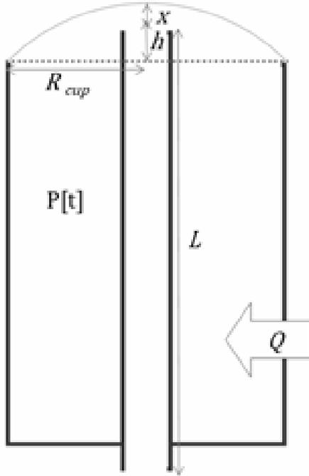
FIG. 4. Drawing of cross-section of the airhorn, with key parameters labelled
