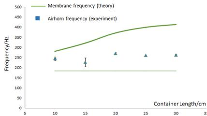
FIG. 11. Frequency of airhorn against length of the container. Light green line represents resonant frequency of the tube
