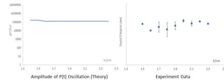
FIG. 12. Sound intensity against height of tube protruding against the membrane ( $h$ )
