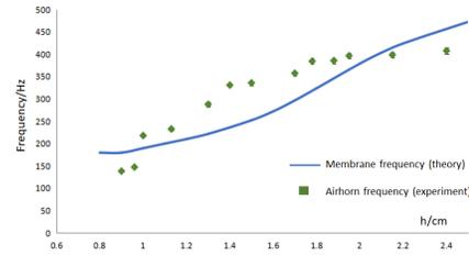
FIG. 9. Frequency of airhorn against height of tube protruding against the membrane ( $h$ )
