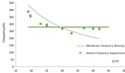
FIG. 10. Frequency of airhorn against length of the tube ( $L$ ). Light green curve represents resonant frequency of the tube
