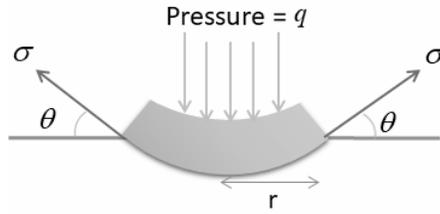
FIG. 5. Cross-section of an infinitesimally small section of the airhorn membrane
