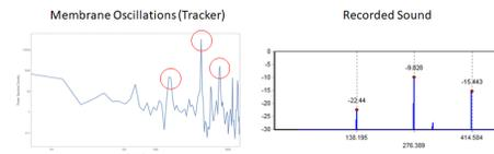
FIG. 3. Fourier transformed plot of membrane oscillation (left, peaks highlighted in red) and the sound produced by the airhorn (right)
