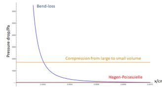
FIG. 8. The three sources of pressure loss plotted against height of the membrane,  $x$
