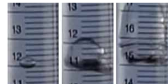
[Fig.3] Bubbles of different sizes rising in a tube. The bubble lengths are 0.23cm, 0.97cm and 2.00cm from left to right, respectively. The diameter of the tube is 1.45cm. The liquid in the tube is water and the tube material is acrylic.
