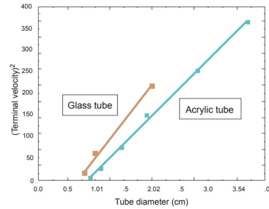
[Fig.7] Effect of tube size on  $V_T$ . The liquid in the tube is water. The tube material is acrylic for the black squares and the formula of the fitting line is:  $V_T^2=128(D_t-0.85)$  with  $V_T$  in the unit of cm/s and  $D_t$  in the unit of cm; The tube material is glass for the red squares and the formula of the fitting line is:  $V_T^2=160(D_t-0.65)$  with  $V_T$  in the unit of cm/s and  $D_t$  in the unit of cm
