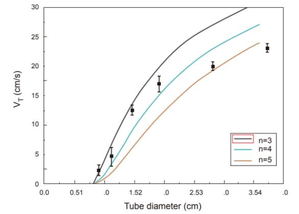
[Fig.8] The effect of tube size on  $V_T$  for the bubbles having the same size. The length of the bubble is about 0.80cm. The liquid in the tube is water and the tube material is acrylic. The black squares are the experiment data. The lines are the fitting curves for [eq.4] changing the tube diameter.  $\rho=1000 \text{ kg/m}^3$ ,  $Re=(10^2, 10^3)$ ,  $R_b=0.4\text{cm}$ . The graph shows that [eq.4] is a good approximation in the range where  $n=3$  to  $n=5$ .
