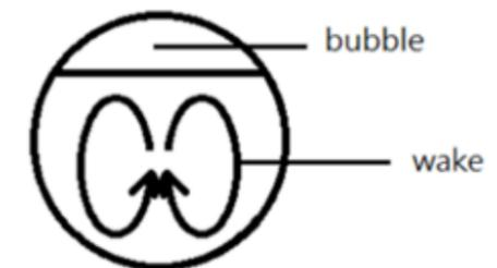
[Fig.14] A diagram that shows the wake behind a bubble. [Ref.1] shows that the bubble becomes non-spherical when  $Re > 1$ .
