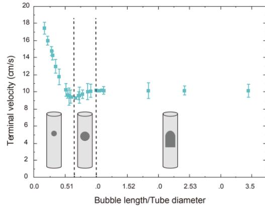
[Fig.5] Effect of  $r$  on  $V_T$  in three regimes. The diameter of tube is 1.45cm. The liquid in the tube is water and the tube material is acrylic. The Reynolds number of the bubbles are between 100 and 1500.
