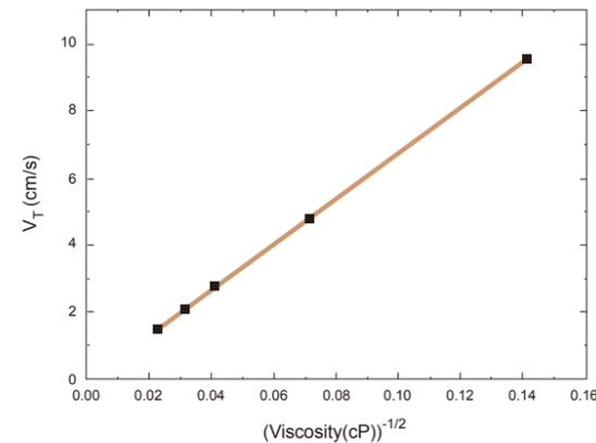
[Fig.10] Effect of liquid viscosity on  $V_T$  of a Taylor bubble. The diameter of tube is 1.45cm. The tube material is acrylic. The liquid in the tube is silicon oil. The formula of fitting line is  $V_T = 70\mu^{-0.5}$ , where viscosity is in cP and  $V_T$  is in cm/s.
