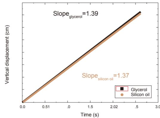
[Fig.9] Influence of liquid property with fixed viscosity on  $V_T$  of a rising bubble. The liquids are glycerol ( $\mu \approx 945 \text{ cP}$  in  $25^\circ\text{C}$ ) and silicon oil ( $\mu \approx 1000 \text{ cP}$  in  $25^\circ\text{C}$ ) for the black line and red line, respectively. The bubbles are Taylor bubbles. The diameter of tube is 1.45cm. The tube material is acrylic.
