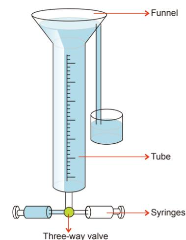
[Fig.2] Experiment setup
