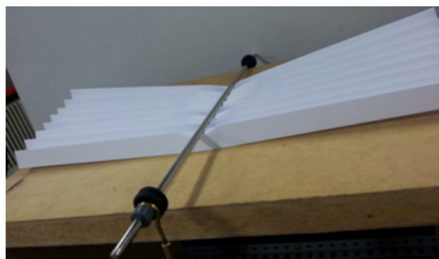
Fig. 5: Local deformation of a truss, due to the ultimate compressive limit.
