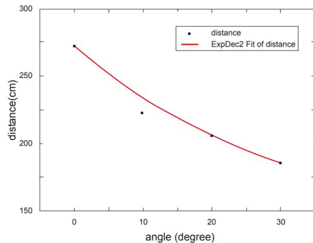
Fig. 5: Distance the car travel change with angle(by experiment) (radius of balloon is 6.75cm, radius of vent is 0.5cm)
