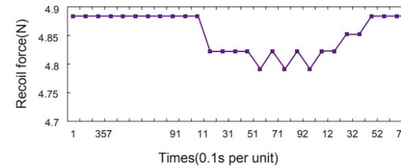
Fig. 2: Recoil force change with time (radius of vent is 0.5cm, radius of balloon is 6.75cm)
