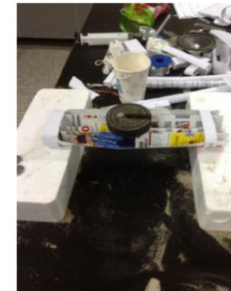
Fig.2 This is a bridge in copperplate paper, it is stronger than printing paper, so it is in good condition under one weight.
