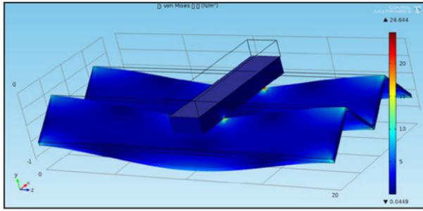
Fig. 3 The simulation based on "Commsol", to analyze the weakest part of the accordion style bridge.
