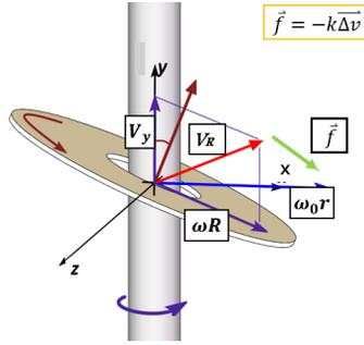
FIG. 3. Diagram of dynamic analysis of ring motion on shaft.  $v_y$  is the component of the ring in the  $y$  direction.  $R\omega$  is the linear velocity of the ring rotating along the axis of symmetry.  $\omega_0 r$  is the shaft rotation speed.  $v_R$  is the total velocity of the ring.  $\vec{f}$  is the wet friction caused by the velocity difference.
