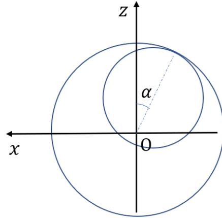
FIG. 2. A schematic diagram of the contact point between the ring and the shaft as a generalized coordinate. It is side view. The big circle represents the inner circle of ring. The little circle represents the shaft. It is the angle between the line connecting of two center and the vertical direction.
