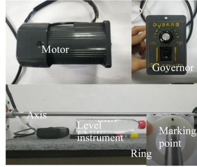
FIG. 4. Image of the experimental device for the motion of the ring on the shaft.
