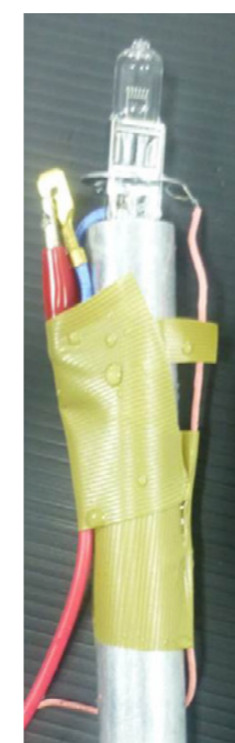
Figure 4: The “fake” candle: candle replaced by a light bulb
