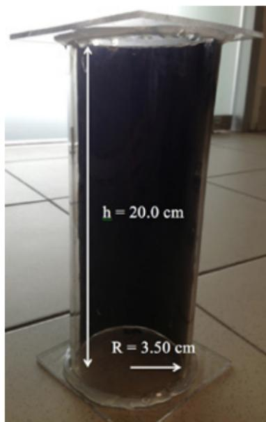
Figure 3.1.1: Cylindrical jar used for investigation. The jar was constructed with acrylic.
