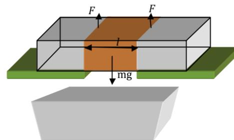
FIG. 10 The experiment setup to measure the adhesion force caused by liquid bridge
