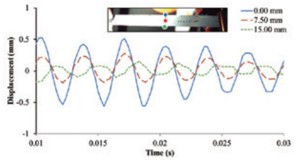
Fig.8. Torsional motion of 10.0 cm by 1.5 cm paper. The points at 0.00 mm, 7.5 mm and 15.00 mm oscillate out of phase as predicted, due to the rotation of paper in this second degree of freedom.
