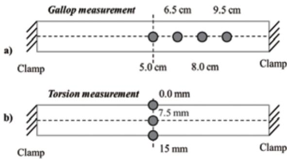
Fig.4. Paper strip (10 cm by 1.5 cm, 70 gsm) schematic of points selected to study a) gallop and b) torsion. Note the actual displacement is the vector sum of both gallop and torsion, but the in-phase / out-of-phase motions reveal the two modes clearly.
