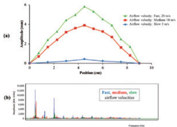
Fig.11. Empirical results of increasing airflow velocities for 9.0 cm by 1.5 cm, 500gsm paper at 5.9 N. Blue, red and green plots correspond to the fast (~20 m/s), medium (~10 m/s) and slow (~5 m/s) airflows. (a) Higher airflow velocities correspond to larger amplitude of oscillation but has (b) negligible effect on frequency spectrum.
