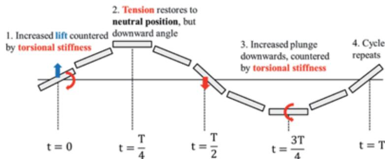
Fig.2. Proposed mechanism for paper strip flutter. Note a common frequency is expected for both torsion and gallop modes, with torsion ahead of gallop, due to the coupled motion
