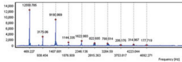
Fig.5. Typical frequency spectrum recorded digitally after FFT, with a paper strip of 8.0 cm by 1.5 cm, 70 gsm and under 6.9 N tension. While 1<sup>st</sup> harmonic (469 Hz) is dominant, a 3<sup>rd</sup> harmonic (1407 Hz) peak exists as well (arb. units on y-axis).
