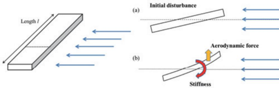
Fig.1. Paper strip cross-section under initial excitation
