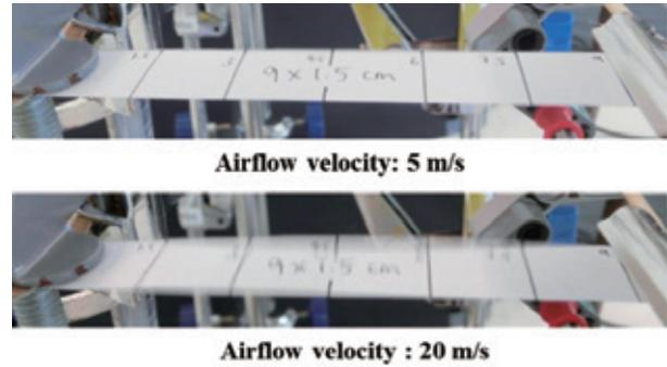
Fig.10. Experiment photographs of larger flutter envelope at higher airflow velocities
