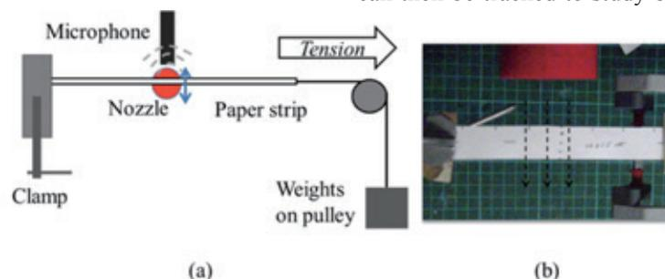
Fig.3. Experimental setup for sound measurement (a) schematic (b) photo. Both ends of the paper strip are firmly clamped to ensure uniform tension, and the nozzle is 3D printed to deliver laminar airflow.
