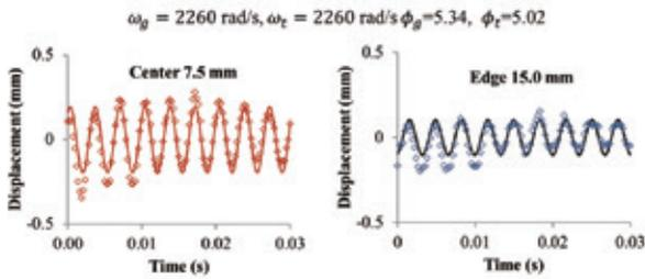
Fig.9. Experimental fitting of paper motion to obtain the angular frequencies and phase constants.
