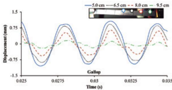
Fig.7. Time domain result of lengthwise motion of 10.0 cm by 1.5 cm paper. The points at 5.0, 6.5, 8.0 and 9.5 all oscillate in phase, with 5.0 cm graph having the largest amplitude.
